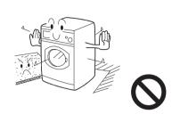
11. During installation, ensure that the electric cable is not trapped by the washing machine and avoid damage to the electric cable. Dear customer, For the machine and your own security, DO NOT REPAIR IT BY YOURSELF! DO NOT USE THE WASHING MACHINE WHICH SOME PARTS ARE LOST!
